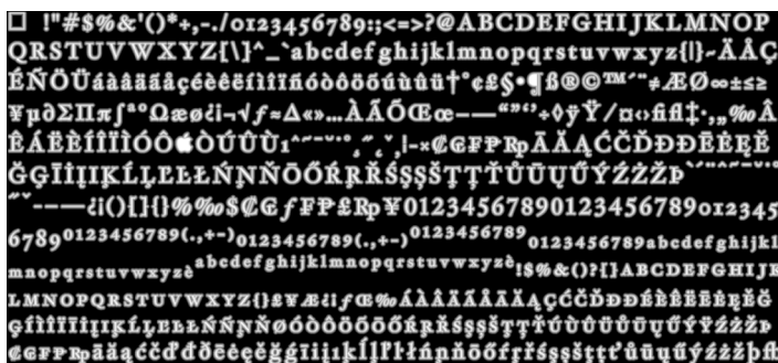
Figure 12.5: The signed-distance field generated from a font atlas. The brightest pixels are the farthest inside.
