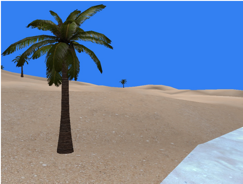
Figure 10.1: The sample app demonstrates alpha testing and alpha blending
