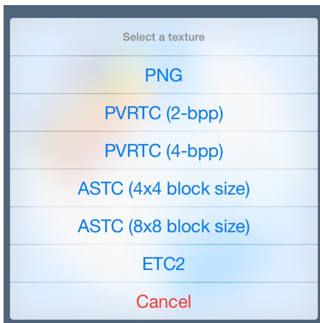
Figure 9.3: The sample app allows you to select among several compression formats supported by Metal.
